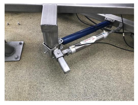
During initial installation you should choke up the clevis as close to post as you can and/or go by feel. Activate the tire shine function and check for pullback clearance off belt. You should have at least 2" from outer edge of belt to brush. If more clearance is needed slide the clevis further out on the arm.
